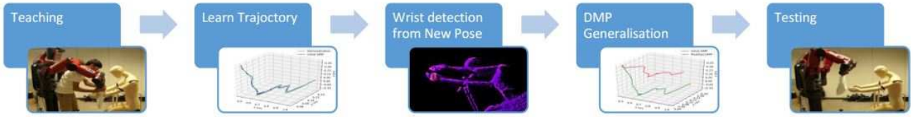
Fig.2: Workflow of robotic cloth manipulation task. Initially, a kinesthetic demonstration is performed with the robot controlled in gravity compensation mode. This demonstration is recorded and parameterized by DMP. Later on, posture of the mannequin is changed. Hand location is detected by Kinect sensor. Accordingly start and goal parameter of initial DMP are modified. Now, the modified DMP can accommodate new posture.
