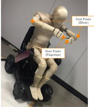
Fig. 4: Control points for arm dressing task showing start and goal points of DMP system colored as orange.
