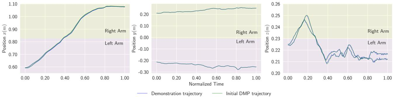
Fig. 6: Baxter’s arms trajectories for both the arms which are parameterized by using DMP. The time is normalized to  $[0, 1]$  range. The figure shows the DMPs are well capable of learning the complex Baxter trajectories.
