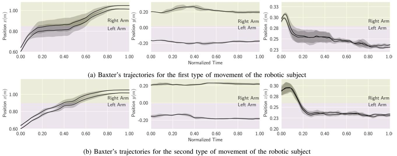
Fig. 8: The trajectories of Baxter's arms for the motions of the robotic subject. Baxter is run ten times for each type of movement. The time is normalized to  $[0, 1]$  range. For each trajectory, the mean position is plotted with the black color, and the region  $\mu \pm \sigma$  along the mean position is filled with the gray color.
