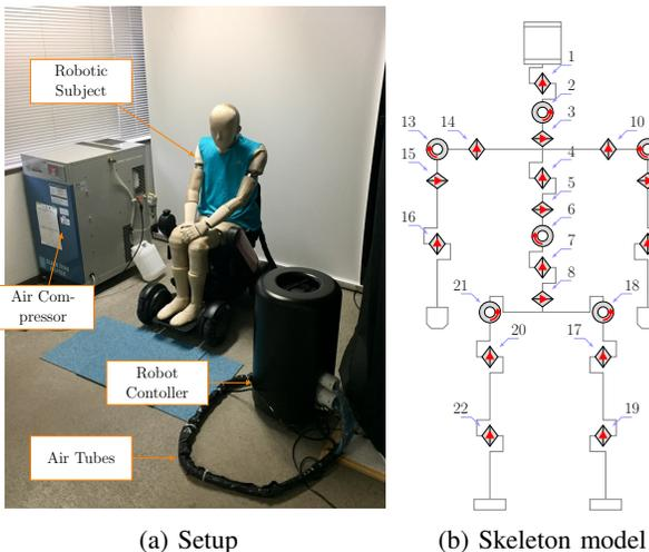
Fig. 2: The robotic subject. Fig. (a) shows all components of the system, Fig. (b) shows the skeleton model of the robotic subject that contains active and passive joints. However, only active joints are shown. All the joints are revolute joints.
